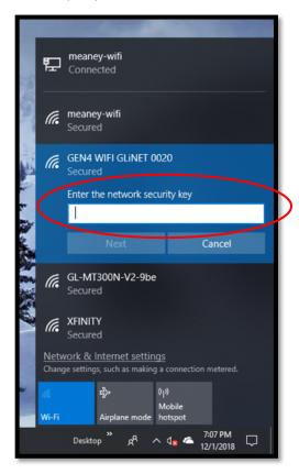
**Step 2.6** - Type the **GEN4** Wireless Network Security Key (Password) under the Enter the network security key dialogue box as shown below and highlight and left mouse click on **Next**.
