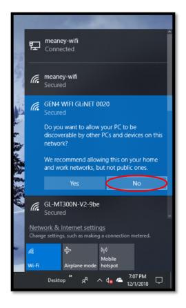
**Step 2.8** - Once **No** is selected from Step 2.7, the following window will open showing your specific GEN4 WIFI GLiNET (0001 thru 9999) network is **Checking network requirements** and is attempting to establish a wireless connection with the PC.
