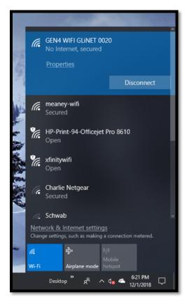
Once the Wireless Network Connection has been established as detailed in Steps 2.0 thru 2.9, an initial online communication can be established between the PC running the BCP software and GEN4 PRO XTREME ECU connected to the GEN4 WIFI GLINET (0001 thru 9999) or GEN4 WIFI NETGEAR (0001 thru 9999) wireless router.
