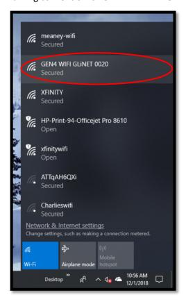
**Step 2.4** - Once the GEN4 WIFI GLINET Wireless Network dialogue window opens as shown below, check the **Connect automatically** box and then left mouse click on **Connect**.
